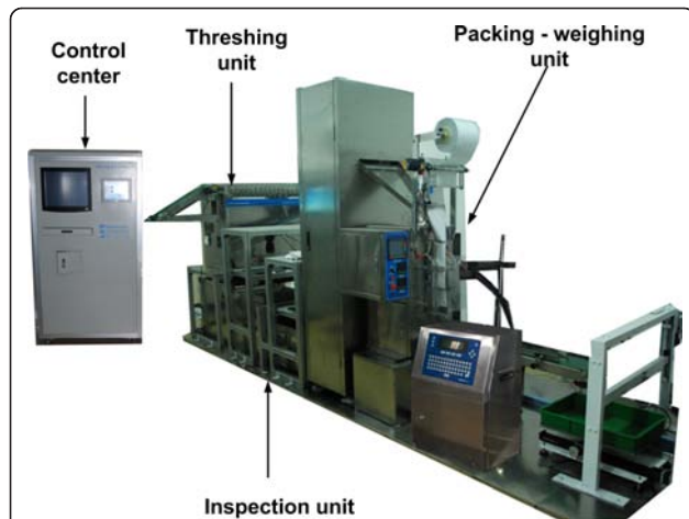
Figure 2 The developed prototype of the SEA facility. The facility mainly consisted of three units: a threshing unit for removing spikelets from the panicles, an inspection unit for assessing and measuring yield traits, and a packing-weighing unit for packing and weighing filled spikelets.
